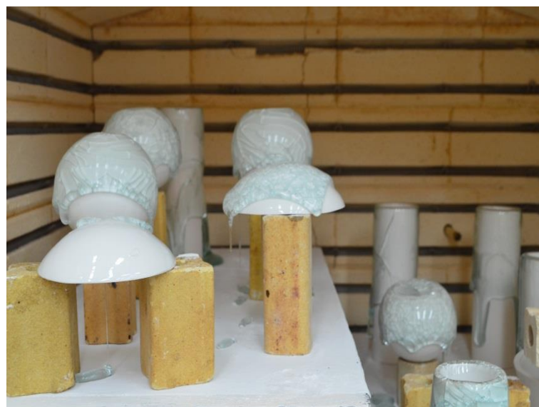
Figure 6 Result of glass melting at 900 degree with same size of glass on different shape of ceramic.
