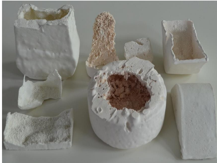
Figure 1 Result of combine porous solid material and clay from dipping technique at 800 and 1200 degree.
