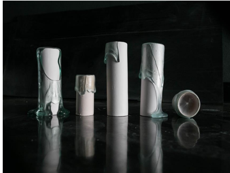
Figure 5 Result of glass melting at 900 degree with same thickness on the same shape of ceramic but different size.
