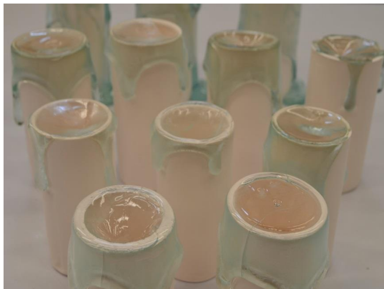
Figure 4 Result of glass melting at 900 degree with same size glass on the same shape of ceramic but different thickness.
