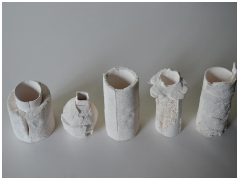
Figure 2 Result of combine porous solid material and clay to texturing the ceramic shape from casting mold technique at 1200 degree
