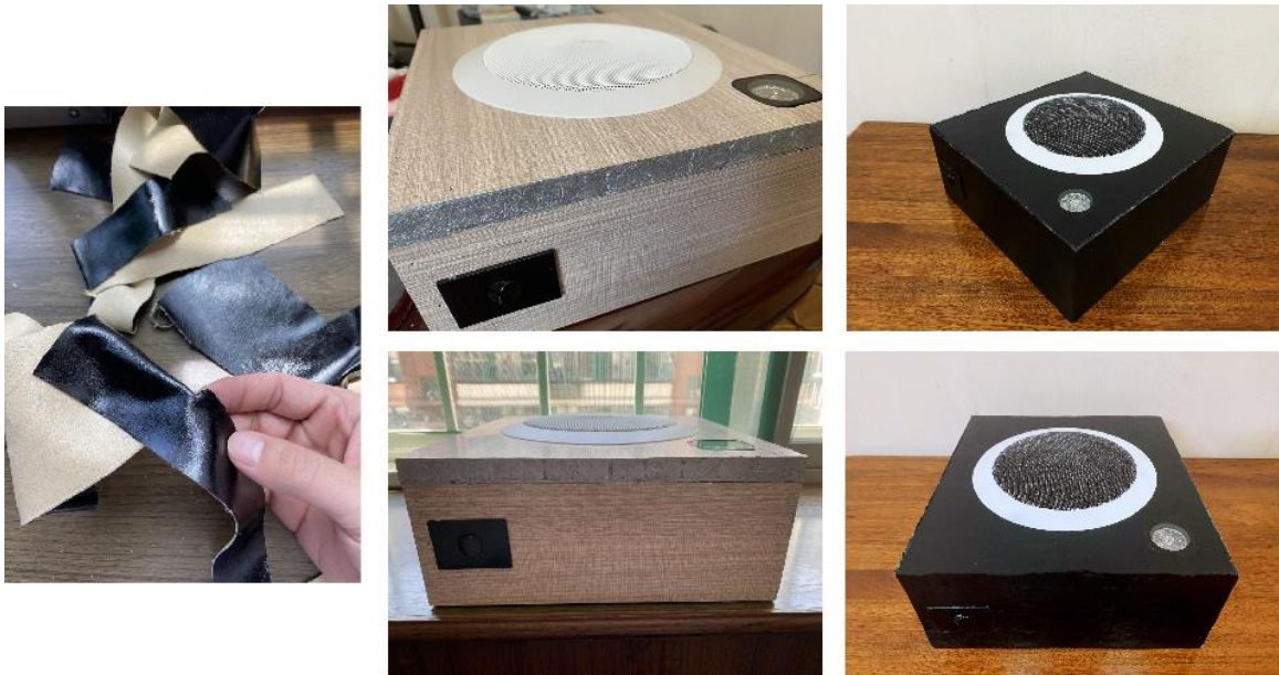
Figure 3.2 The physical object after wrapping the leather
