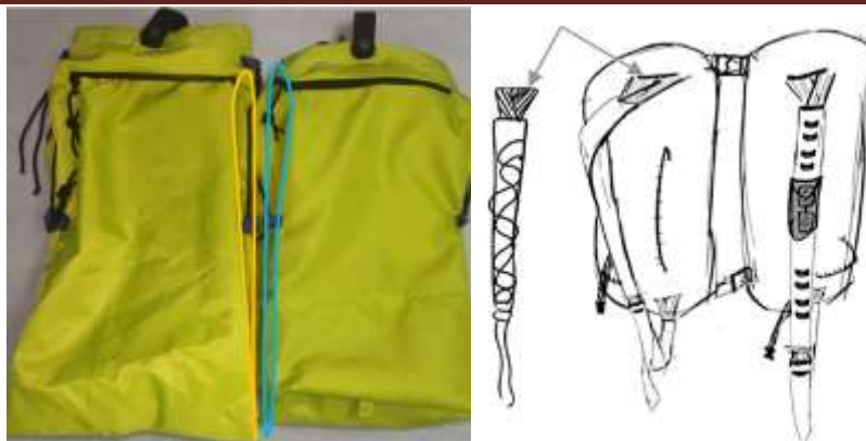
Figure 11 Place Velcro in the orange and blue labeled areas to act as a hold on the backpack(left);
